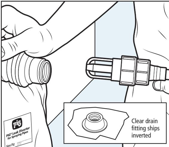
1. Identify and invert the clear drain fitting in the middle of the unit so the fitting is on the outside of the unit with external threads exposed. Install hose adapter.
